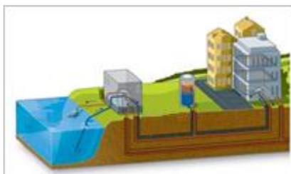
heat and up to 20 MW cooling. The heat source for the heat pumps is sea water extracted in 30 meters depth approximately 400 meters out in the fjord. By relying on sea water for both,
