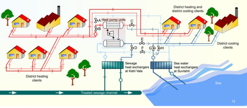
Thus, the Unitop<sup> $\circ$ </sup> 50FY heat pumps are able to produce the full temperature lift required. The chilled water produced is absorbed completely by the district cooling system. During times without heat load, the condensing temperature is lowered to match with sea water conditions and the heating energy is rejected to the sea, resulting in a very high COP. (Valves A + H open, Valve B + C closed, Valves E + F open, Valves D + G closed).
