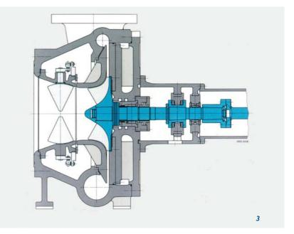
A flexible coupling is connecting the compressor with the high efficient gear and the driving motor.
